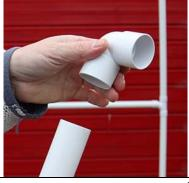
TWIST AND SECURE THE 90 **DEGREE BENDS ONTO** EACH END OF THE REMAINING 1270MM PIPE
