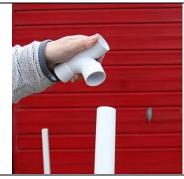
CONNECT TEE JOINT TO 1270mm length of PIPE
